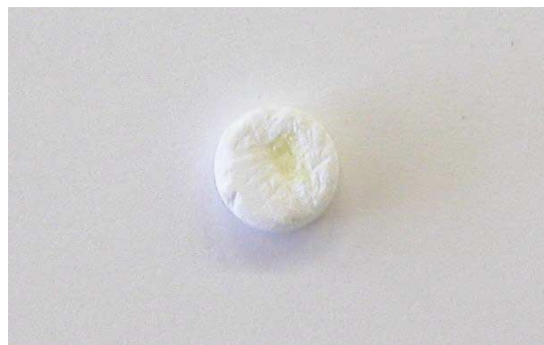
Fig.1 Photograph of Contaminants on Tablet
