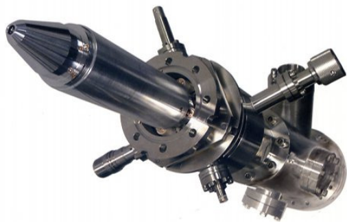
Figure 2 Multi-mode gas cluster ion source.
