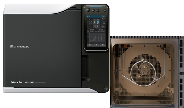
Fig. 1 Appearance of Nexis™ GC-2030 and Example of Glass Column Installation
