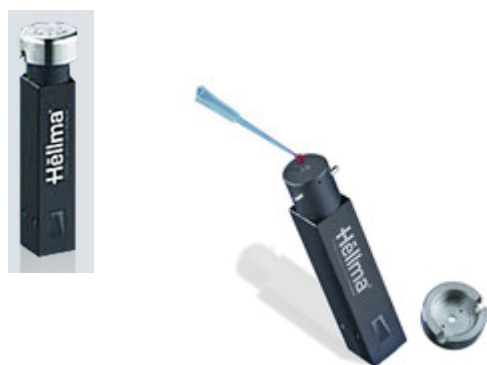
Fig. 1 Photograph of TrayCell and Sample Pipetting
