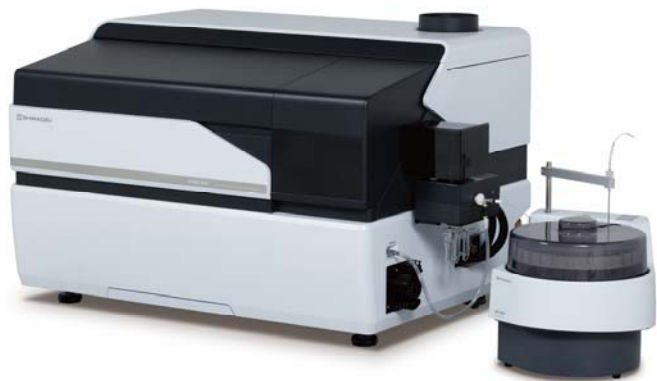
Fig 1. Shimadzu ICPMS-2030 with autosampler AS-10 Continuous Calibration Verification (CCV) checks were run in between to monitor drift of the system throughout the run. Standard of LOQ concentration was run as CCV.
