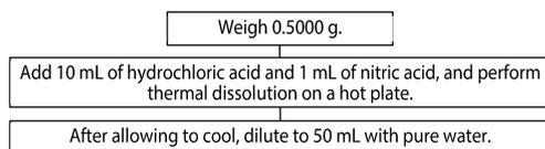
**Fig. 4 Acidic Dissolution Procedure**
