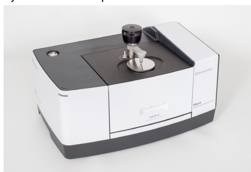
Fig. 1 External Appearance of IRSpirit™ + QATR™-S
