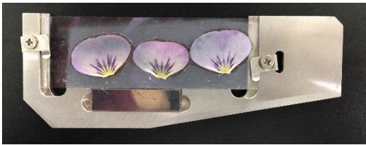
Fig. 3 Samples Mounted in Dedicated Holder (ITO Slide Glass)
