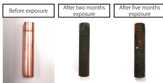
Fig. 2 External appearance of copper pipe before and after corrosion
