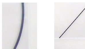
Fig. 1 Appearance of Sample Materials (Left: ① Nylon 6 + Short Fiber CFRP, Right: ② Nylon 6 + Continuous Fiber CFRP)
