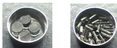
Fig. 2 Sampling Conditions (Left: Short Fiber, Right: Continuous Fiber)
