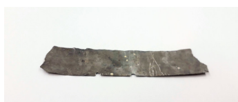
Sheet-shaped cadmium (Cd) 1.2 × 11.8 cm
