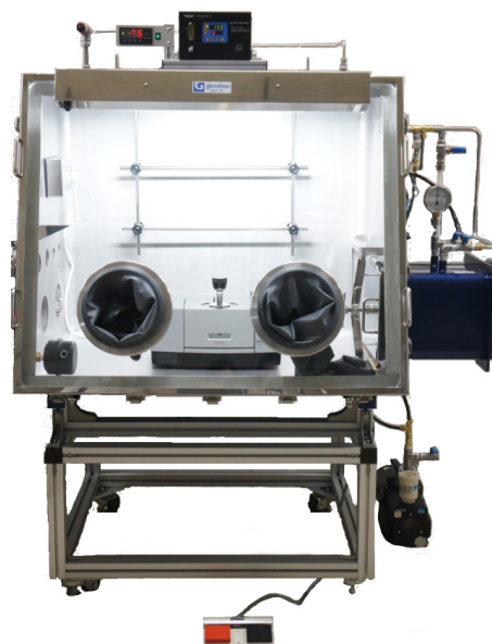
Fig. 2 Example of IRSpirit Glove Box System
