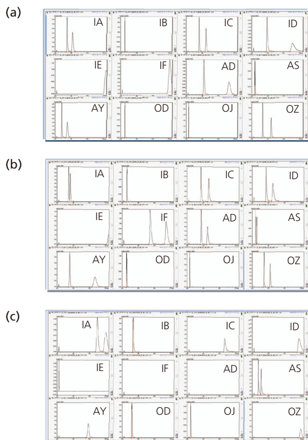
Fig. 36 Chiral Screening Separation Results Modifiers: (a) Methanol, (b) Ethanol, and (c) Acetonitrile/ethanol = 75/25 (v/v)
