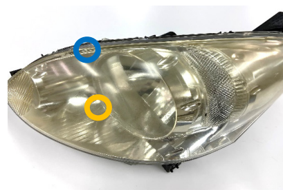
Fig. 2 Measurement Specimen (Yellow Circle: Yellowed Part, Blue Circle: Transparent Part)
