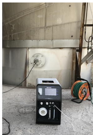
Fig. 2 Condition of CO Concentration Measurement by CGT-7100
