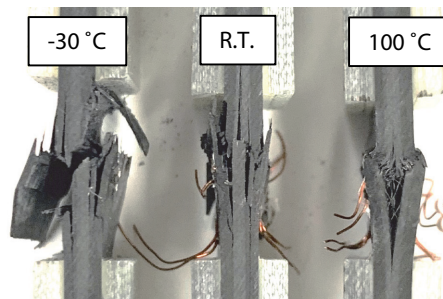
Fig. 8 Fracture Condition in Evaluation Area of Test Specimens ( -30^{\circ}\text{C} , R.T., 100^{\circ}\text{C} )
