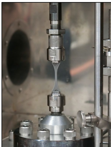
Fig. 3 High Speed Tensile Test
