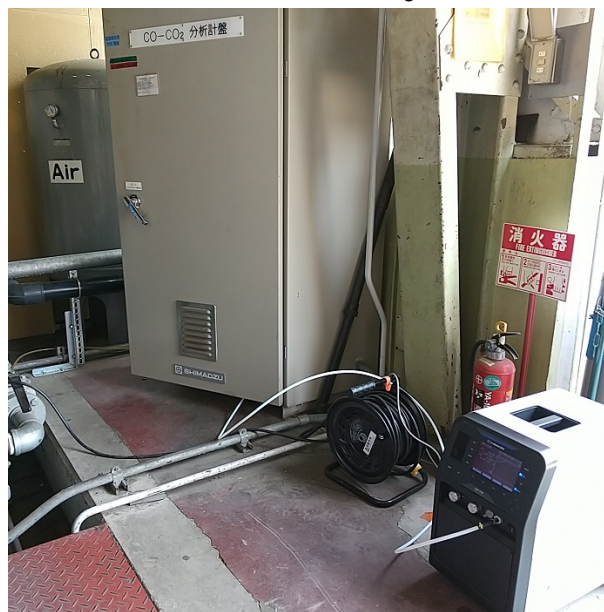
Fig. 5 View of CGT-7100 Taking Atmosphere Measurements from a Carburizing Furnace
