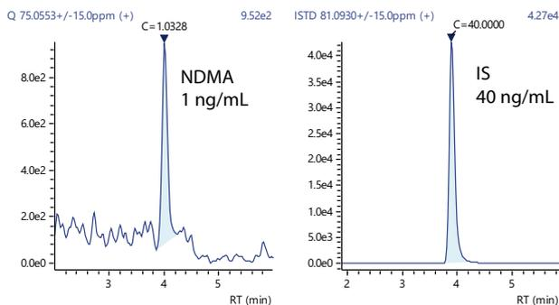
**Figure 2** XICs of NDMA of 1 ng/mL and IS (NDMA-d6) of 40 ng/mL.
