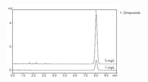
$\begin{array}{lll} \text{System} & : \text{Prominence}^{\text{TM}}\text{-}\text{i} \\ \text{Column} & : \text{Shim-pack GIST C8} \\ \end{array}$
