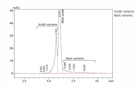
Column : Shim-pack Bio IEX SP-NP (100 mm x 4.6 mm I.D., 3  $\mu$ m), P/N : 227-31005-03
