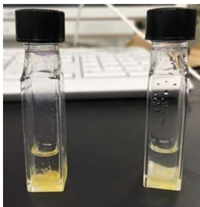
Fig. 3 Appearance of Nylon 6i Resin Used as Specimens. (Left: Without Photo-Irradiation. Right: With Xe-Lamp Irradiation for 6 Hours.)
