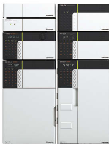
Prominence HPLC with RID-20A for carbohydrate analysis
