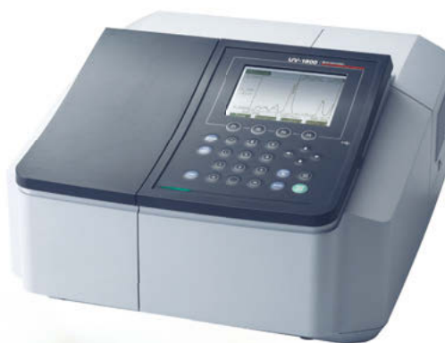
Shimadzu UV-1800 for measurement of beer bitterness and alcohol content
