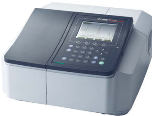
Shimadzu UV-1800 for measurement of beer color
