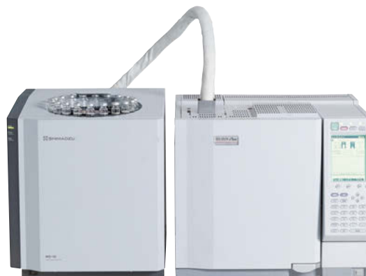
Shimadzu GC-2010 Plus or GC-2014 with HS-10 Headspace Autosampler for analysis of vicinal diketones
