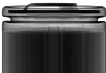
Fig. 2 Fluoroscopic Image of the Positive Terminal in a 21700 Type LIB Cell
