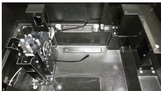
Fig. 2 Installation of the Spectacle Lens in the MPC-2600A Sample Compartment
