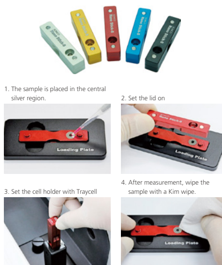
Figure 2 What the Nano Stick Looks Like and How To Use It
