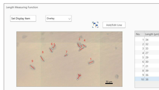
Fig. 6 Operation Screen of Length Measurement Function and Results of Length Measurement
