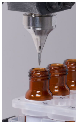
Fig. 4 LotusStream Gas-Liquid Separator
