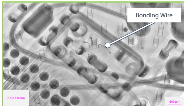
Fig. 7 X-ray Fluoroscopic Image of the Crystal Oscillator
