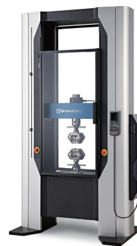
Fig. 31 AGX-V Precision Universal Testing Machine
