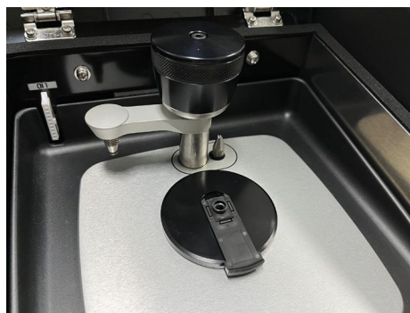
Fig. 2 Specac Arrow accessory on QATR™ 10 ATR accessory
