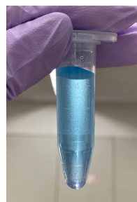
CNF aqueous suspension after 10x dilution of the supernatant
