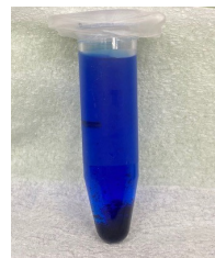
Dye-adsorbed CNF aqueous suspension after centrifugal separation
