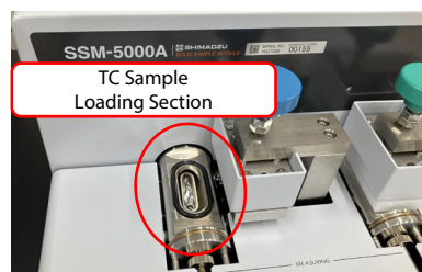
Fig. 4 Sample Boat Set in the TC Sample Loading Section
