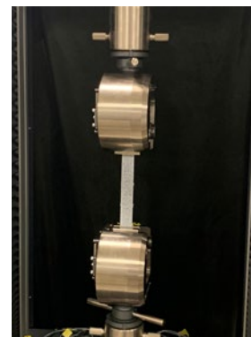
Fig. 3 Wedge Grips for FRP
