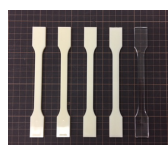
Fig. 1 Appearance of Specimens From left, PC : ABS = 0 : 100, 25 : 75, 50 : 50, 75 : 25, 100 : 0
