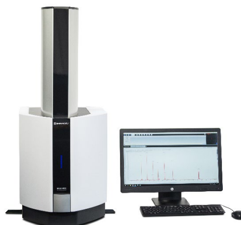
Fig. 2 MALDI-8020 Benchtop MALDI-TOF Mass Spectrometer
