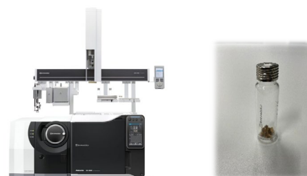
Fig. 1 GCMS-TQ™8040 NX (left) and cigarette leaf sample (right)
