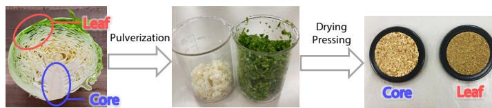
Fig. 1 Outline of Sample Preparation Procedure
