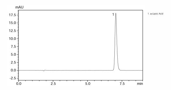
Column Shim-pack VP-ODS (150 mm x 4.6 mm I.D., 5 μm), P/N: 228-34937-91 Shim-pack GVP-ODS (10 mm x 4.6 mm I.D., 5 μm), P/N: 228-34938-91\* Guard Column Mobile phase 10 mmol/L (Sodium) phosphate buffer (pH 2.6) / Acetonitrile = 6 / 4 (v/v)
