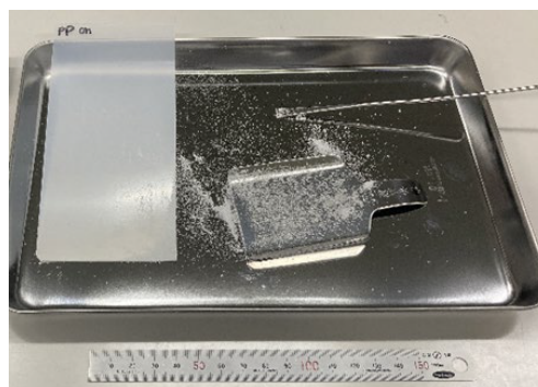
Fig. 4 Preparation of PP Microplastic Particles
