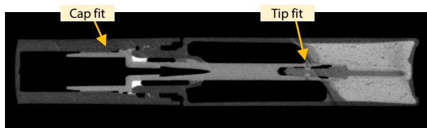
Fig. 6 Cross Section of the Liquid Lipstick
