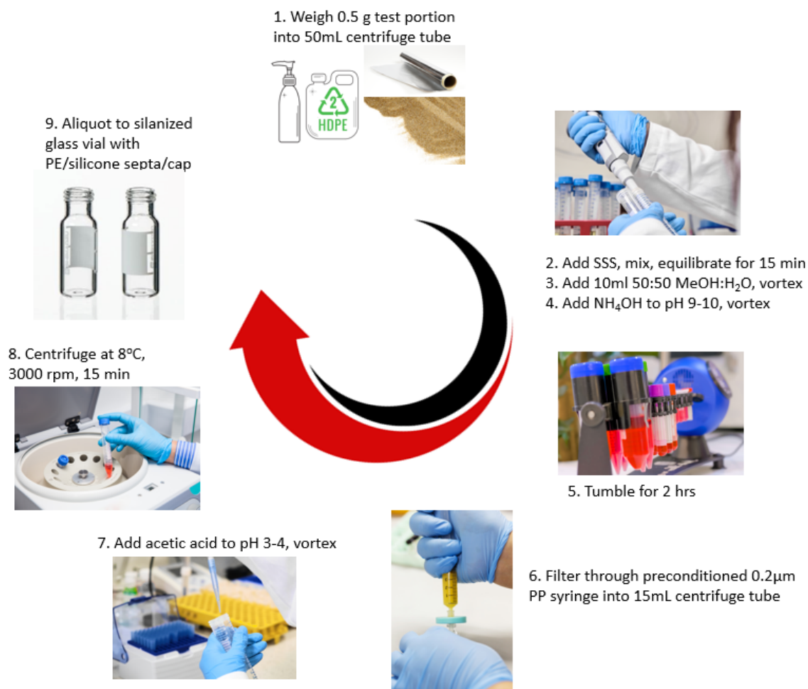
Fig. 2: Sample preparation procedure for consumer products
