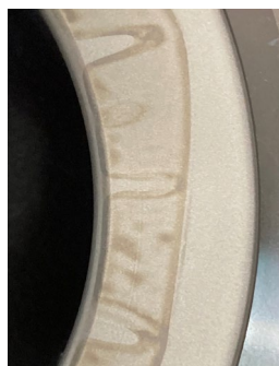
Fig. 1 Brown Stain Adhered on the Surface of the Circular Workpiece
