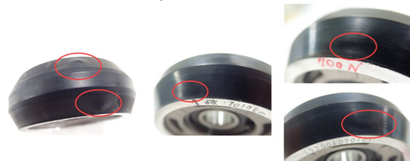
Fig. 3 Workpiece Bulges (Left: 2 Locations on Workpiece A, Center: 1 Location on Workpiece B, and Right: 2 Locations on Workpiece C)
