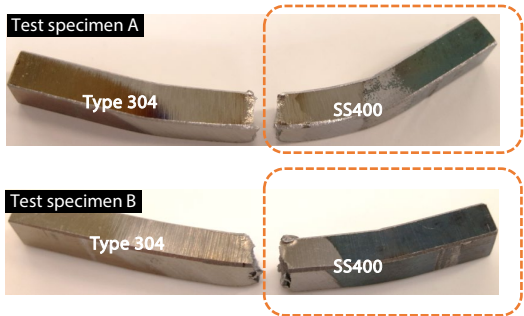
Fig. 6 Test Specimens A and B after the Fatigue Tests
