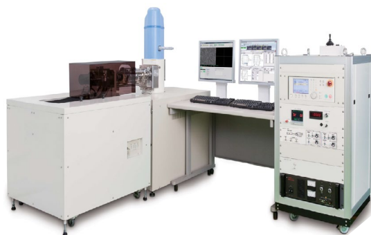
Fig. 1 Servopulser with Scanning Electron Microscope
