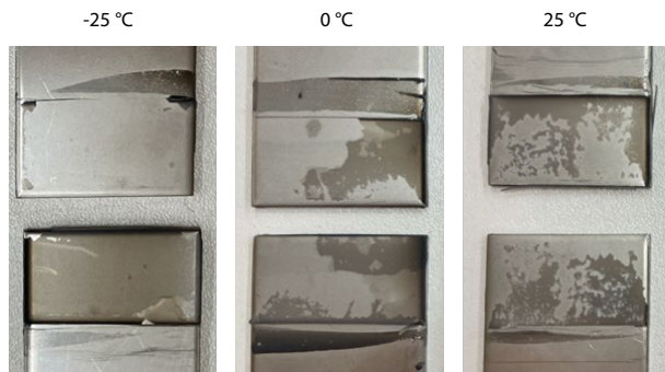
Fig. 5 Fracture State of TB2049/2149 at -25 °C, 0 °C and 25 °C
