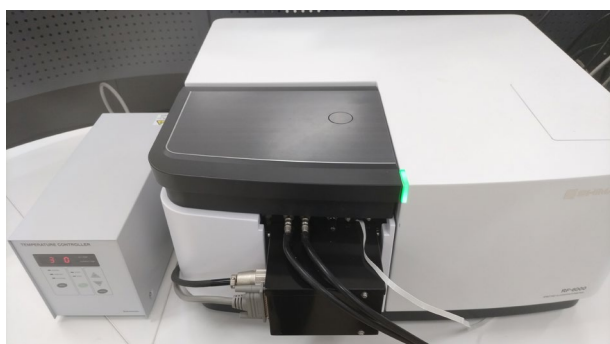
Fig. 1 RF-6000 Spectrofluorophotometer with Thermoelectric Single-Cell Constant-Temperature Holder
