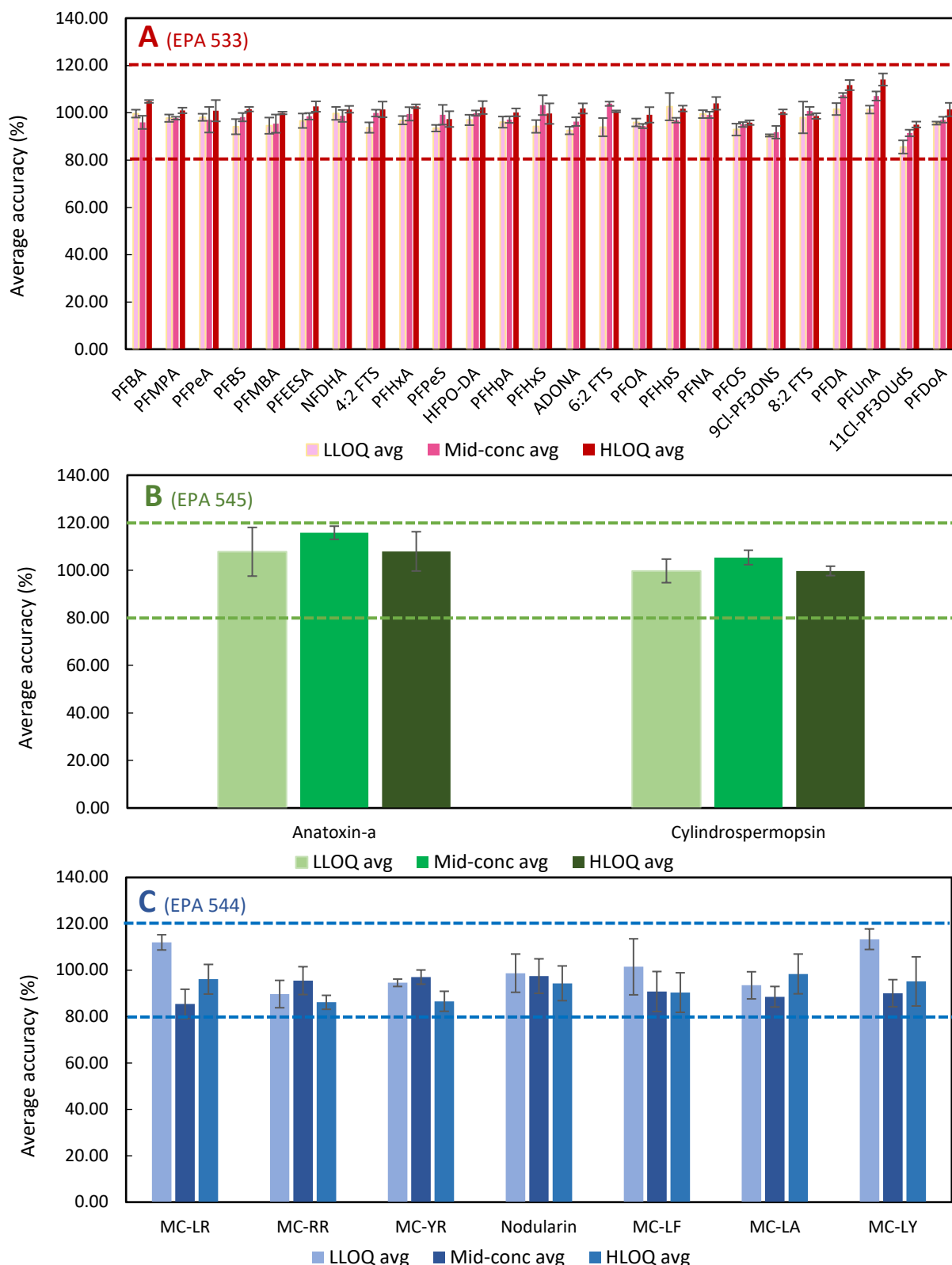
Figure 6: Results of continuing calibration checks for the three EPA methods. A: EPA Method 533. B: EPA Method 545. C: EPA Method 544.
