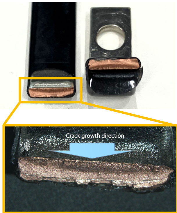
Fig. 12 Fracture Surface Photograph of In-plane 30 N Test
