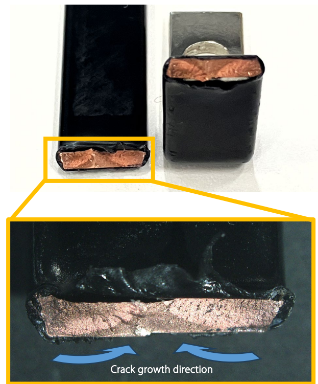
Fig. 13 Fracture Surface Photograph of Out-of-plane 60 N Test
